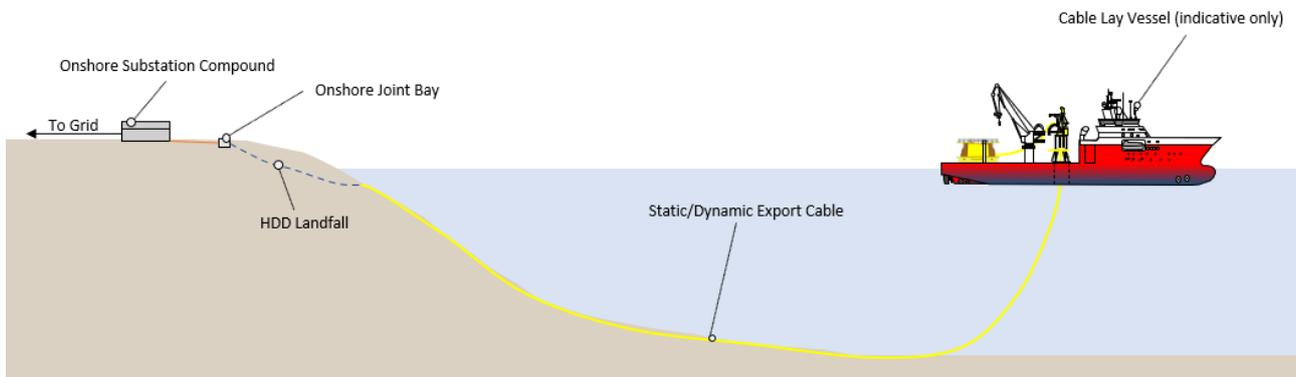
Figure 5.14 Offshore export cable installation
