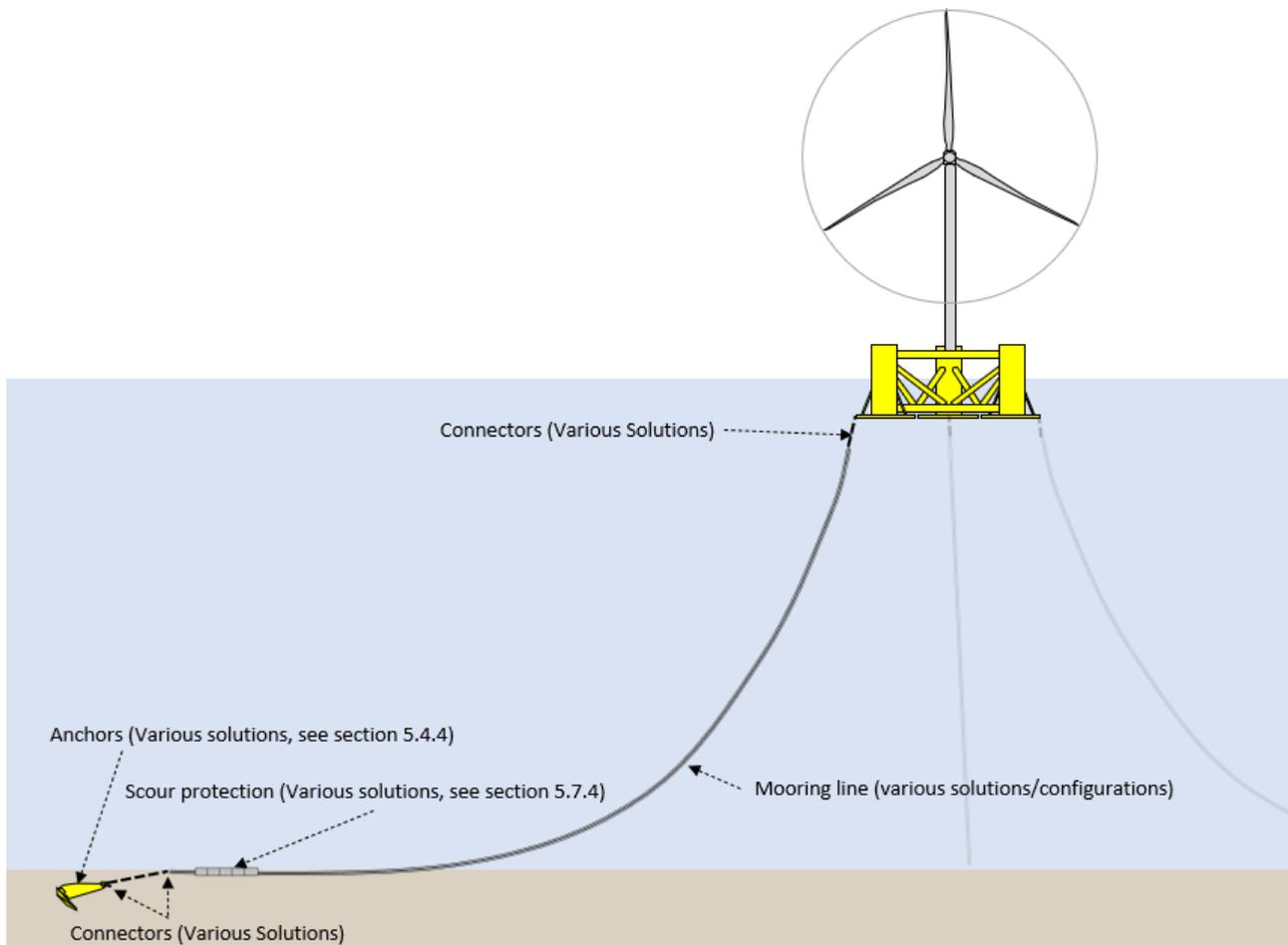
Figure 5.6 Key components of a typical mooring system
