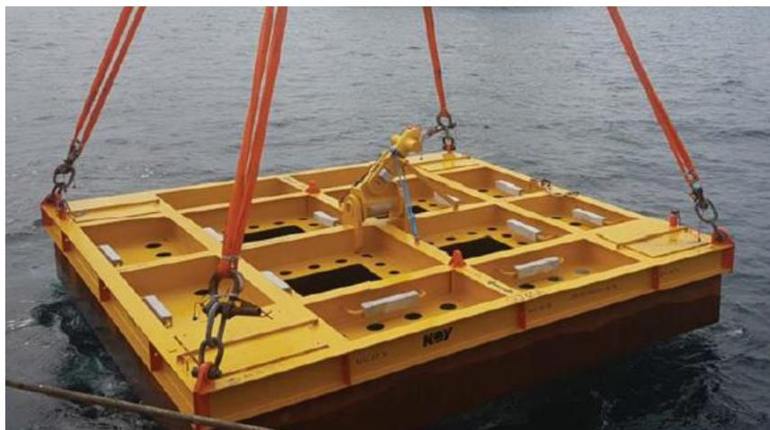
Figure 5.11 Typical anchor structure to be deployed on inter-array cables
