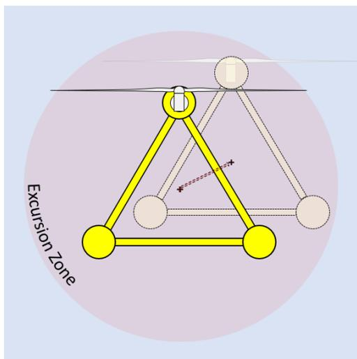
Figure 5.8 Floating structure excursion (illustration)
