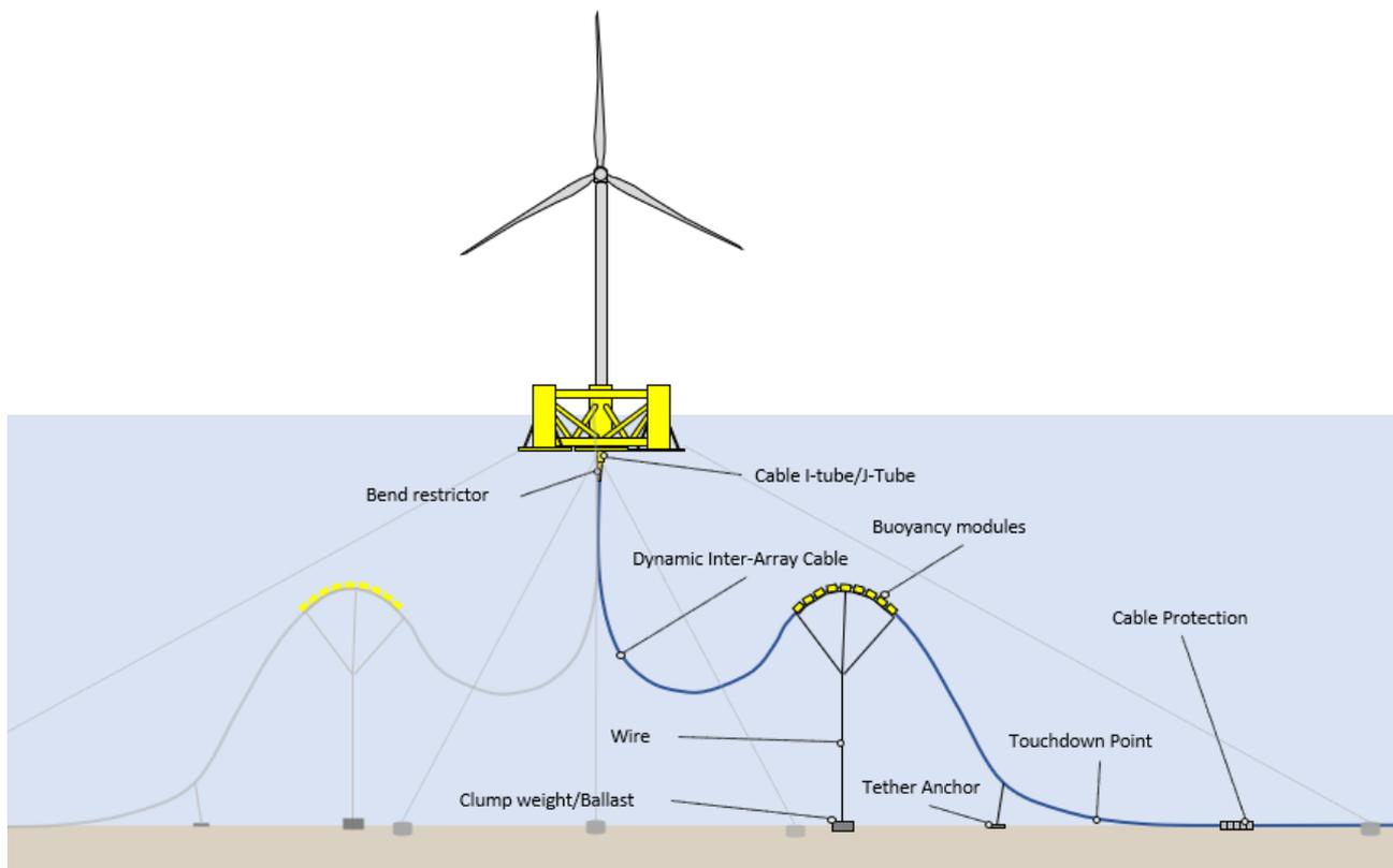
Figure 5.9 Typical dynamic cable arrangement
