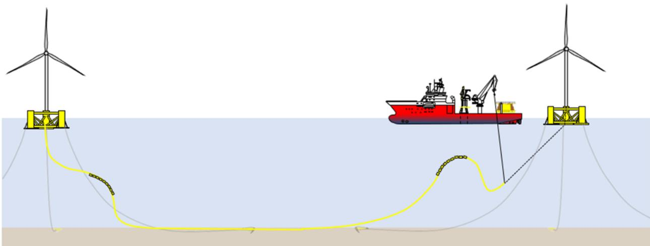
Figure 5.13 Inter-array cable installation (including catenary mooring for illustrative purposes)
