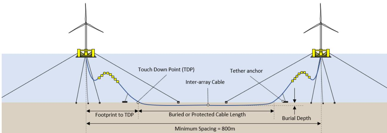
Figure 5.10 Dynamic inter-array cable dimensional characteristics (for illustrative purposes)
