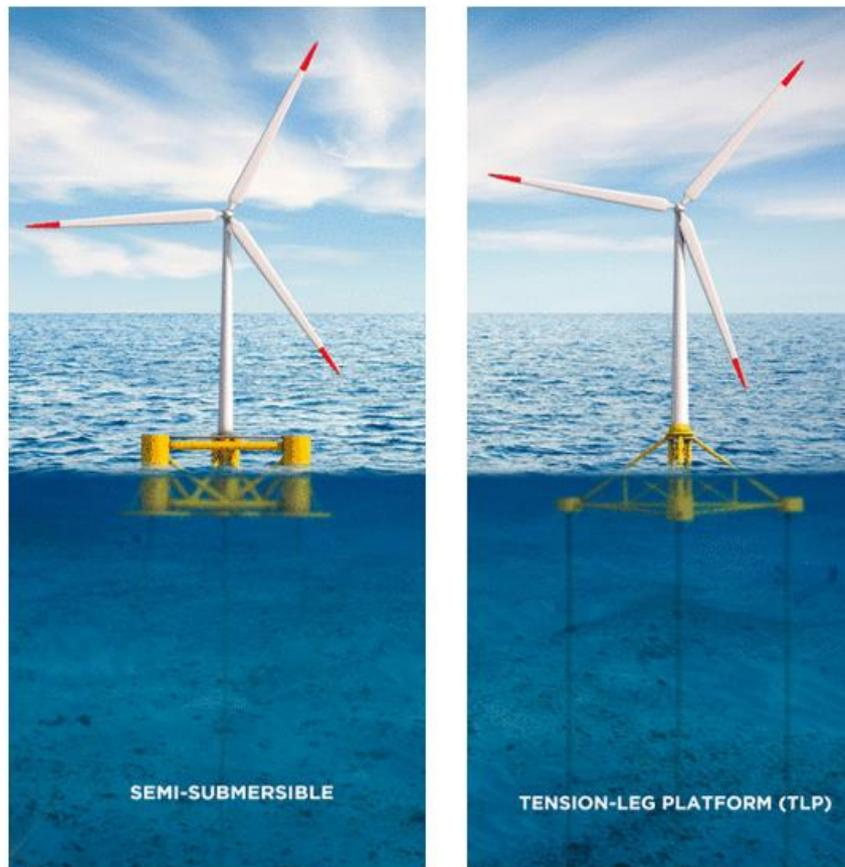
Figure 5.4 Illustration of characteristic floating substructure designs (Image from WindEurope)
