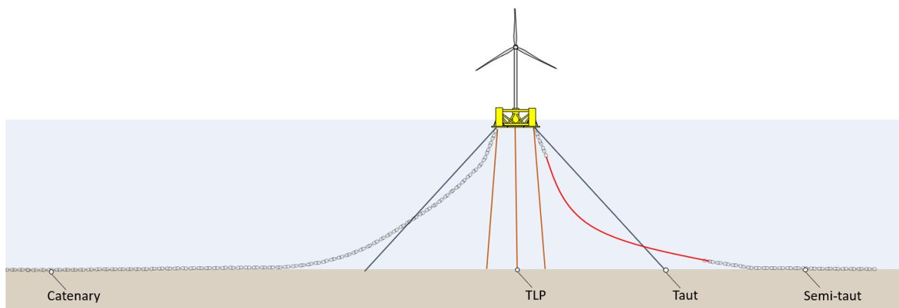
Figure 5.5 Illustration of potential mooring system configurations
