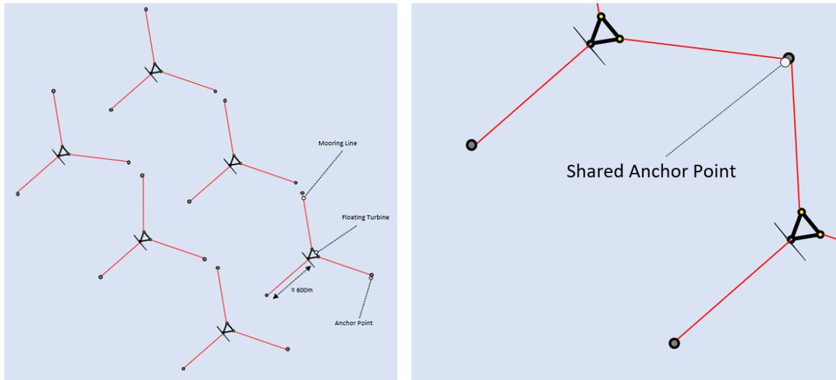
Figure 5.7 Example of a typical mooring layout (left) and shared anchor point (right)
