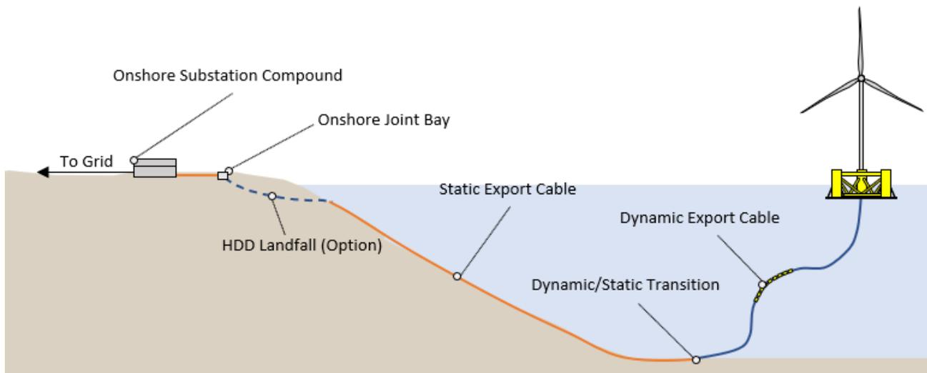
Figure 5.12 Key elements of a floating wind farm offshore export cable
